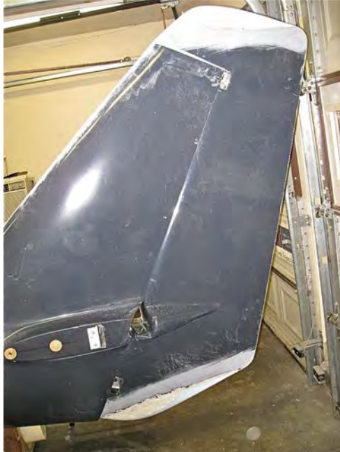
Pic #78 shows again my final rudder re-shaping of the top and bottom, a strictly cosmetic change to suit my preferences.
