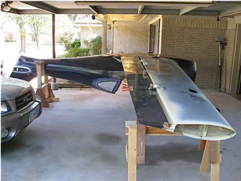
Photo #175 shows the wings being drilled for the angle of incidence bolts. My carport sure came in handy for this, since the plane was outside for several days.
