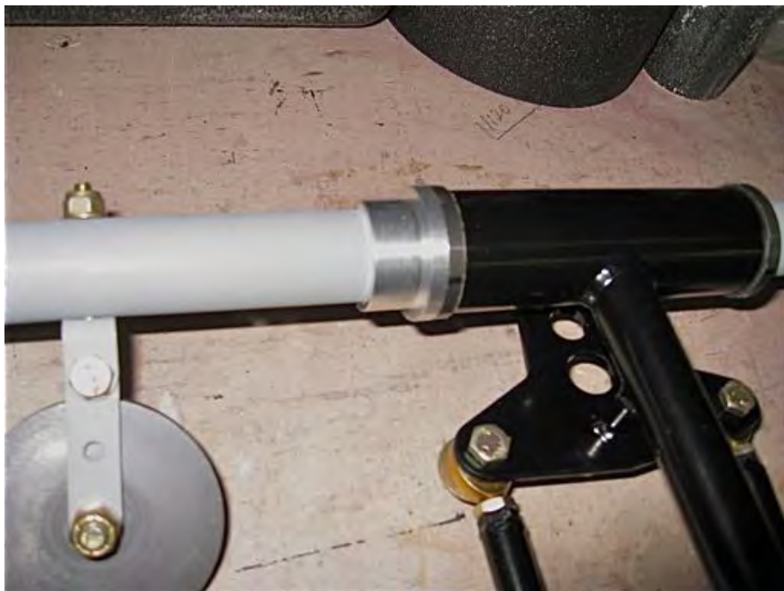
Photo #148 shows some support bushings that a friend machined for me. I liked this better than using a short section of the split 1" aluminum tubing at this location.
