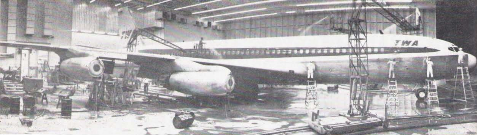
A wash job for a big jet plane calls for a vast room, barrels of detergent and water by the thousands of gallons. This is standard procedure at TWA's overhaul base.
