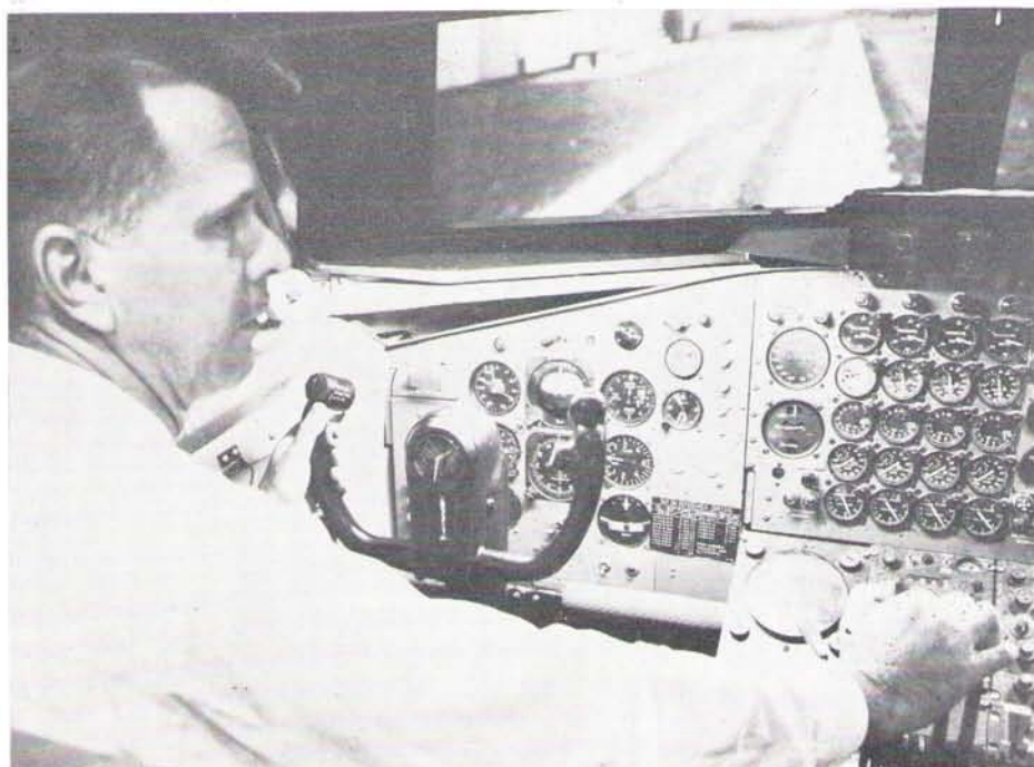
Closed circuit television projects airport scene on a large screen in front of the pilot's cockpit to give greater realism while training at TWA's Jack Frye International Training Center.
