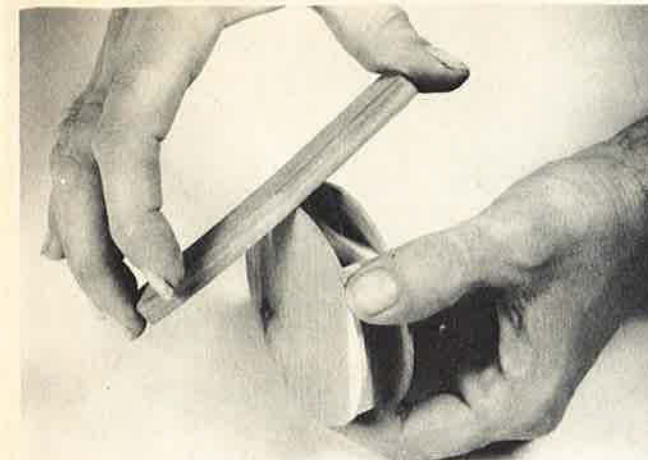
One must make certain that the "sound holes" or slots are of suitable size in each end of box when completed.
