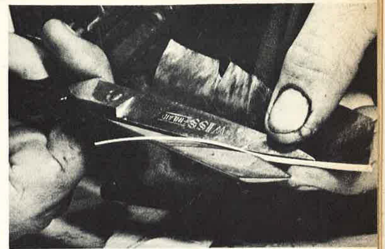
3. The width of the quill also is checked. If the widths do not match up, this is easily remedied with a pair of scissors. Cut the quill base to get same widths for quills.
