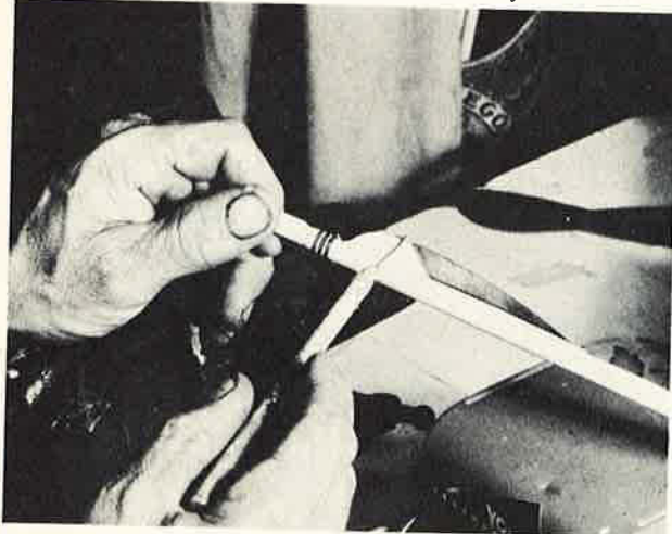
14. After the fletch has been burned, the mounted needle can again be brought into play, using it to remove the rough edges. Fine grade sandpaper also may be used.
