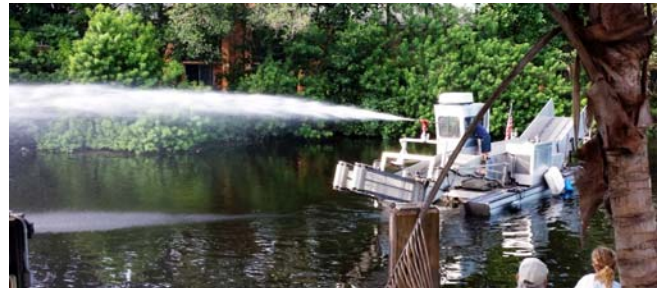
The high pressure nozzle flushes debris out from under docks.
