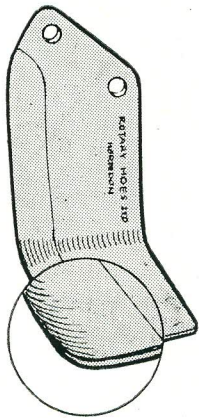
Fig. 4 Enlarged view of blade with cutting edge turned inwards
