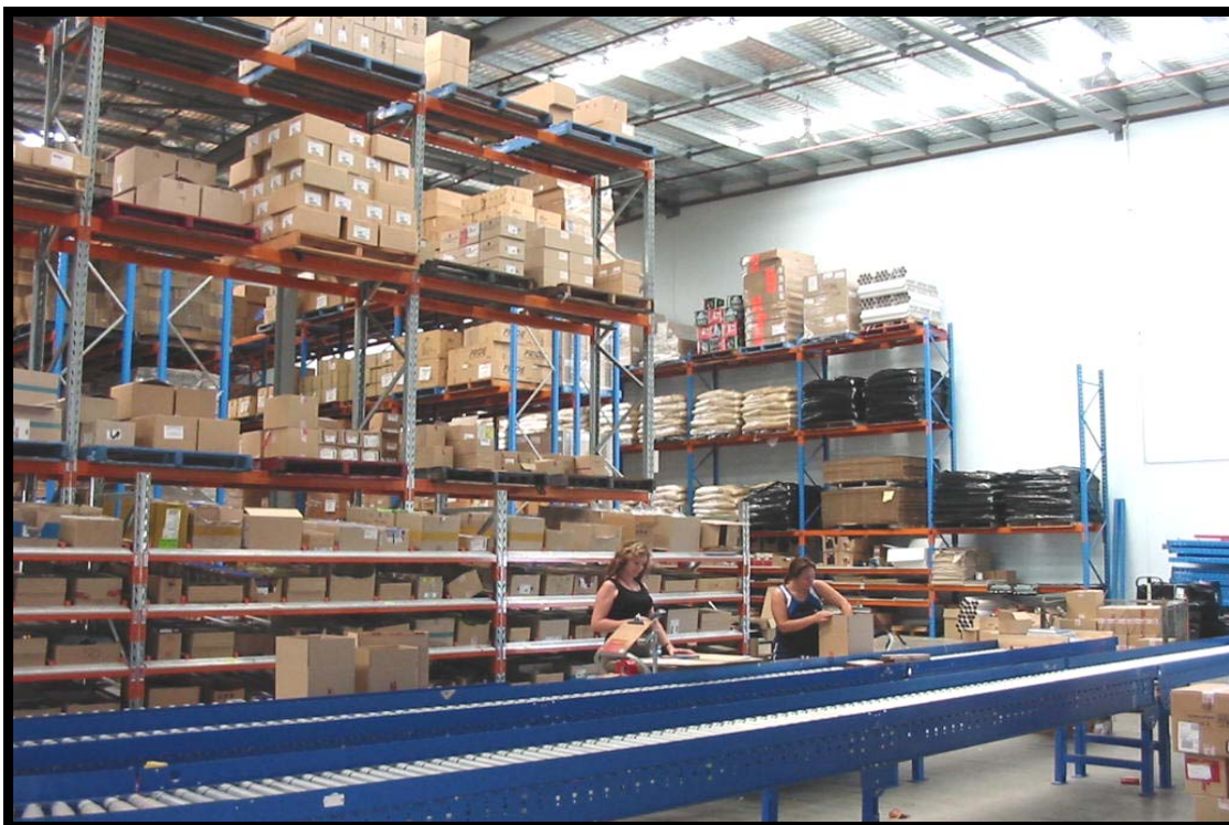
Figure 13 – Open cartons and low level areas not suitable for ESFR
