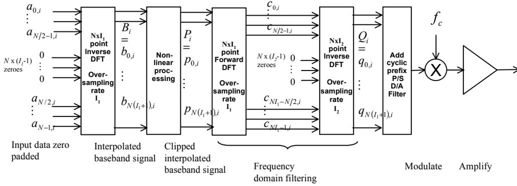
Fig. 1. Block diagram of peak reduction technique
