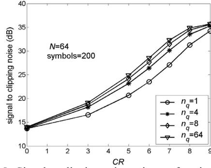
Fig. 5. Signal to clipping noise ratio as a function  $CR$  for varying  $n_q$
