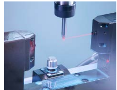
Measurement with laser for determination of the spindle drift at high speed
