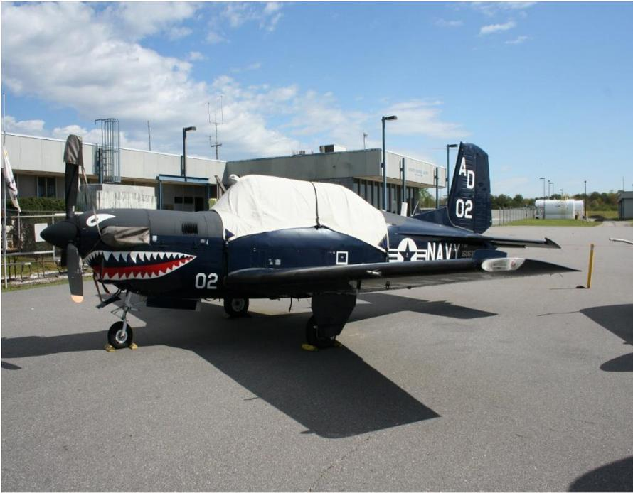
The Beechcraft T-34 Mentor is an American propeller-driven, single-engine, military trainer aircraft derived from the Beechcraft Model 35 Bonanza. The earlier versions of the T-34, dating from around the late 1940s-1950s, were piston-engined. These were succeeded by the upgraded T-34C Turbo-Mentor, powered by a turboprop engine. The T-34 remains in service over six decades after it was first designed.
