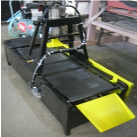
Figure 5. Completed Conveyor Based Can Crusher
