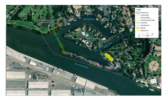
According to the Certification, the Smith Canal Gate Project would also include approximately 1,660 linear feet of continuous floodwall and seismic stability wall along the eastern portion of Dad's Point.(Certification, p. 3.) Recreation facilities would be installed on Dad's Point to replace amenities affected by project construction, such as fishing, wildlife viewing, walking, biking, and running. (*Ibid.*)
