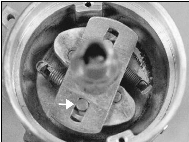
1962/64 distributor design. The fly-weights were directly opposed by spring forces. The cam was advanced as the fly-weight pins moved along slots in the cam (*arrow*).
