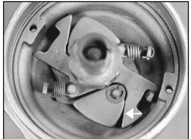
1965/69 distributor design. Fly-weights acted against a changing contact surface (*arrow*) to reduce centrifugal forces acting against the calibration springs.
