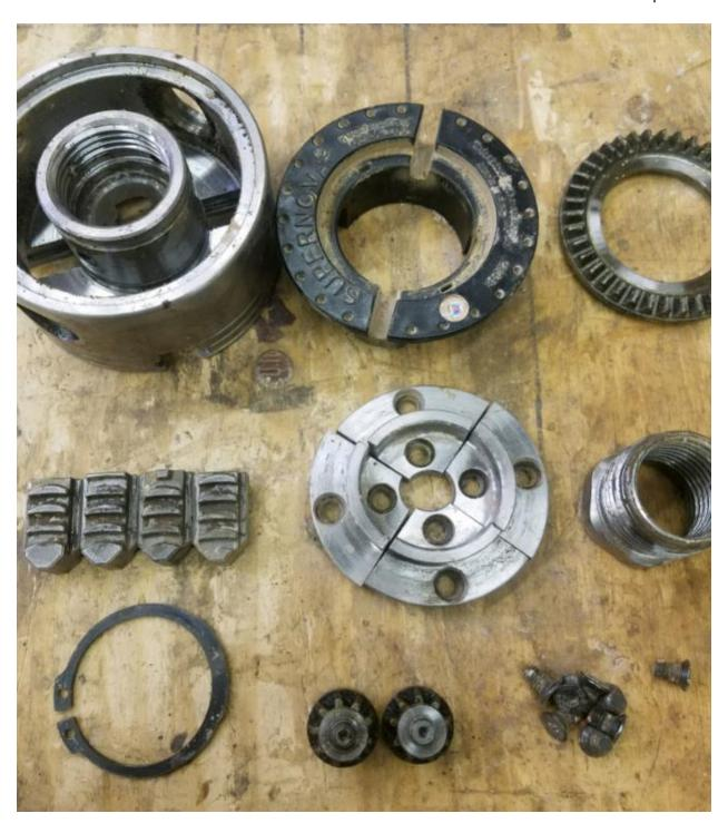
Clean all parts and inspect for damage. Mineral spirits and a toothbrush work well for cleaning. I used emery cloth to remove some of the surface rust caused by green wood. For more challenging rust Home Depot sells a product called Metal Rescue that is amazing for removing rust. A 1 Gallon jug will last for years as it can be reused over and over.
