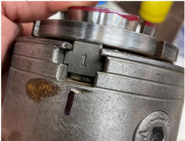
Completely disassemble the chuck as shown in the photos. Once the snap ring is removed the black plastic cover can be a challenge to remove especially if it has been a while since the chuck was cleaned last. Keep at it and it will come out.
