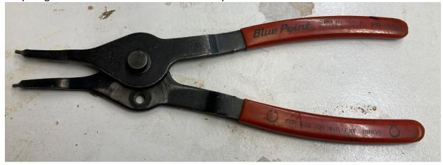
Mark the movable jaws prior to disassembly. It is not always absolutely necessary to return parts to their original position, but it can eliminate potential difficulties. A sharpie will do until you make a permanent mark with a center punch.
