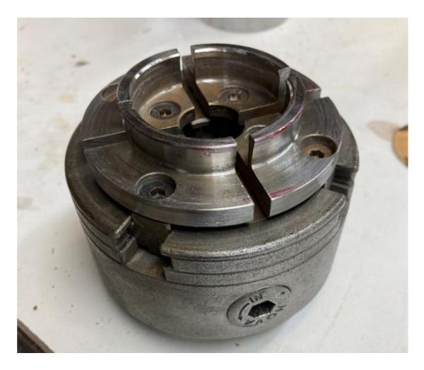
Disassembly requires only one special tool, snap ring pliers. These make removal of the snap ring easier and safer than needle nose pliers.
