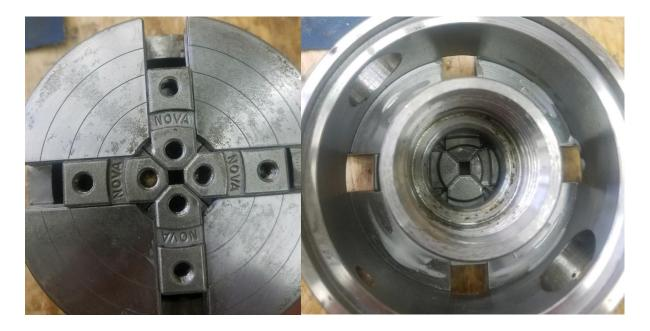
Carefully turn the chuck upside down keeping the jaws from moving, Place the scroll in and rotate it until it engages the jaws. All jaws must move together and close into a square at the center. Pinions and plastic housing are installed then the snap ring.
