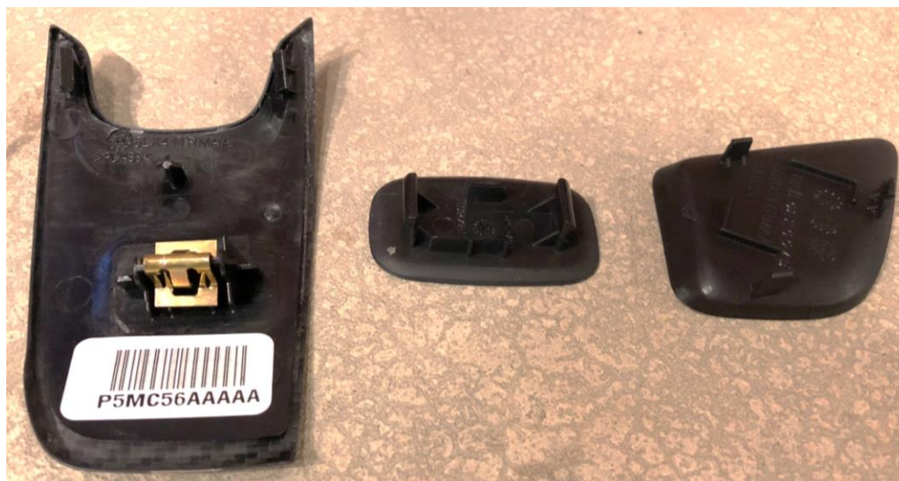
Backside of trim pieces removed to gain access to screws
