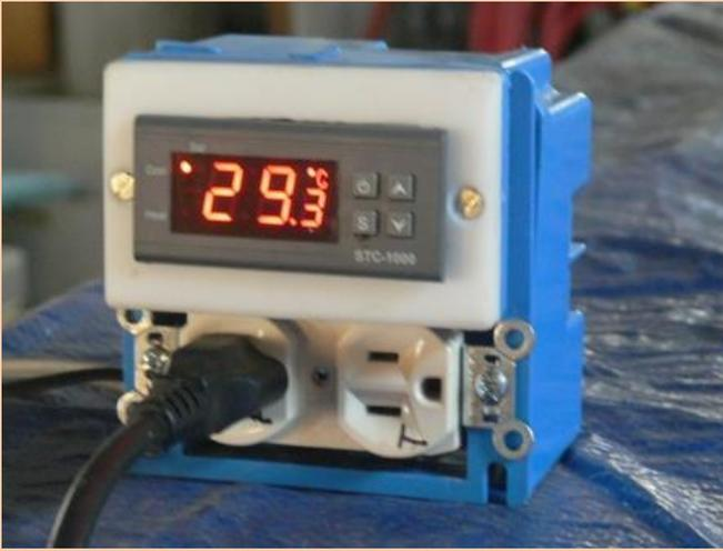
buying one from Hong Kong through EBay, using Pay pal for \$15.00 plus \$10 air mail! It seemed to good to be true but I got it in the ten days and it was exactly what I needed. Has a 10 amp relay for heating and one for cooling. I wired it into a common plastic double outlet box with an outlet. Works perfect! I can't say enough about this
