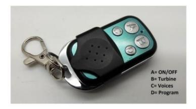
press turbine 1 time= on/off turbine
