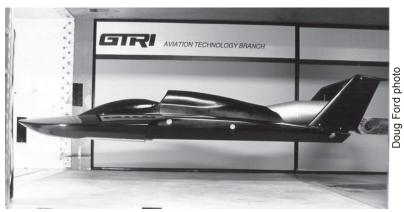
Miss Budweiser T4 in the wind tunnel at GTRI, Aviation Technoligy Branch
