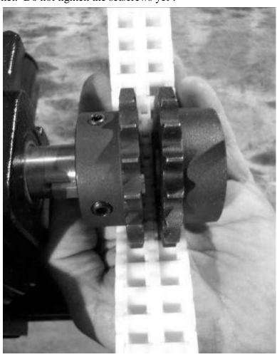
4.) Remove the link pin from the new plastic chain by pulling the "E" clip off either end with needle-nose pliers or similar. Hold the square-bored sprocket in place and wrap the chain around both sprockets. Make sure the chain "meshes" with the teeth on both sprockets, and wraps all the way around until the two end links align, and the link pin can be inserted through them. Carefully reinstall the "E" clip into the groove in the pin.
