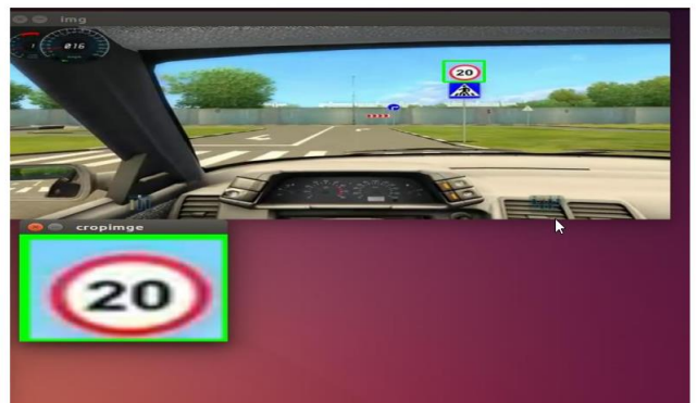
Step 3: symbol recognition and alert will be in the form of buzzer
