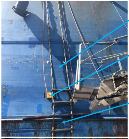
Pilot ladder should extend 2 meters above the lower platform of an accommodation ladder.
