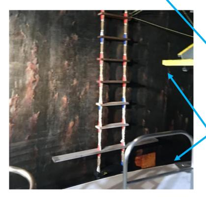
Accommodation ladder should be well secured to the ship's side.
