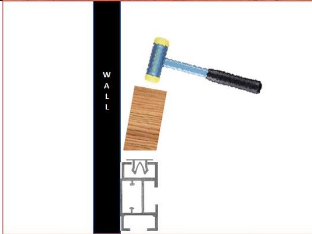
Use a piece of 2" x 4" to inserting the TS79W PVC insert on the side. This way you will get enough space to pound your hammer on the insert. Cut the 2" x 4" with an angle of 15 degrees, it is sufficient to give some space and provide a good transmission of the blow on the insert.
