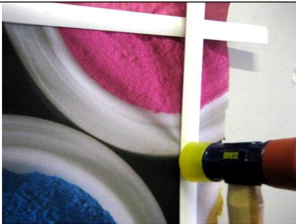
Then the insert segments are removed using a flat screwdriver and replaced by a longer one using a dead blow hammer or a **hard nylon head** hammer.
