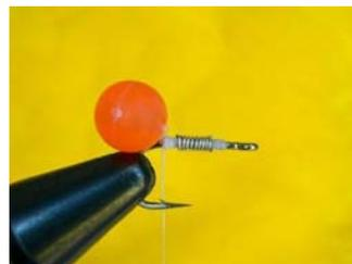
3. Optional - Start the .015 inch lead free wire 3/32 inch in front of the Trout Bead. Take 8 to 10 touching wraps of wire forward to just past mid shank. Cut away the wire tag ends and bind the wire down to the hook shank with back and forth GX2 thread wraps so the wire will not move when the crosscut rabbit strip is applied. When finished binding the wire down the thread will be hanging at the bead tie on point at the back of the hook.
