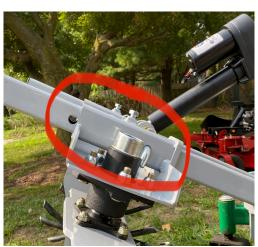
and not tightened. Additionally, you should retorque these bolts after the first use.
