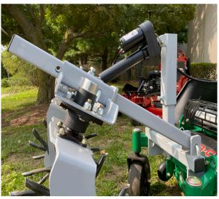
3) **VERY IMPORTANT** When using the ZRator, ONLY APPLY ENOUGH DOWN PRESSURE TO PENETRATE THE SOIL 1-2" (or raise the caster wheels slightly in harder soil conditions). Once the aerator is in motion, it will penetrate enough to pull deeper plugs and you will have the best traction and maneuverability. If you apply too much down pressure (which is not necessary), there will be too much torque and heavy side load resulting in potentially breaking tines.
