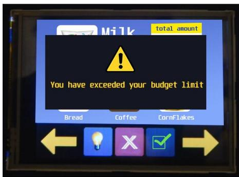
Fig 9: LCD Screen Display: alert on reaching budget limit
