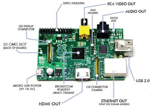
Fig 2: Raspberry Pi with associated components explained
