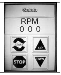
4) Turn ON the refrigeration toggle switch on the right hand side of the machine. Note that the refrigeration WILL NOT start without the beater running!
