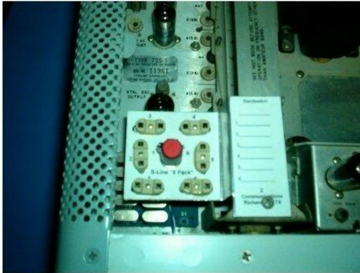
The "6 Pack" installed in a 75S-1
