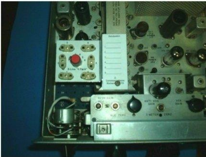
The "6 Pack" installed in a KWM-2A
