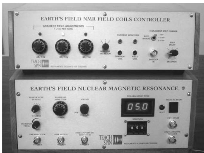
Figure 4: Earth's Field and Gradient Coil Controllers
