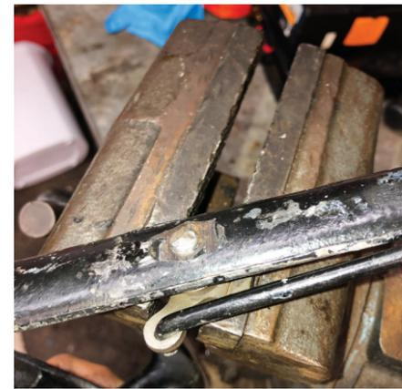
5) Cold peen the head of the rivet to the hand brake lever. Use a secure, hard, and flat surface for backing the larger side of the rivet to secure it.
