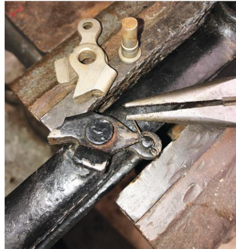
1) First remove the cross shaft from the frame, passing it under the chassis. Then remove the small cotter pin from the hand brake lever rod.
