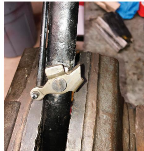
4) Test fit the new ratchet pawl on the new stepped rivet to be sure the action is free; if not, polish or sand the axle portion for smooth operation. A smear of grease on the axle portion of the rivet helps.
