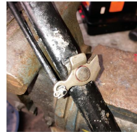
6) Complete the task by fitting the lever rod and inserting the cotter pin, then test the action. The brake handle's flat spring should be in good condition as well. If not, replace it or use the accessory ratchet pawl spring - to fit one of those, open the circle end to wrap around the base of the control cross shaft, clip it shut, and place the hook end on the inside of the lever rod.
