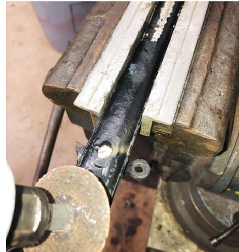
2) Locate the rivet end and grind it down to expose the rivet shaft.
