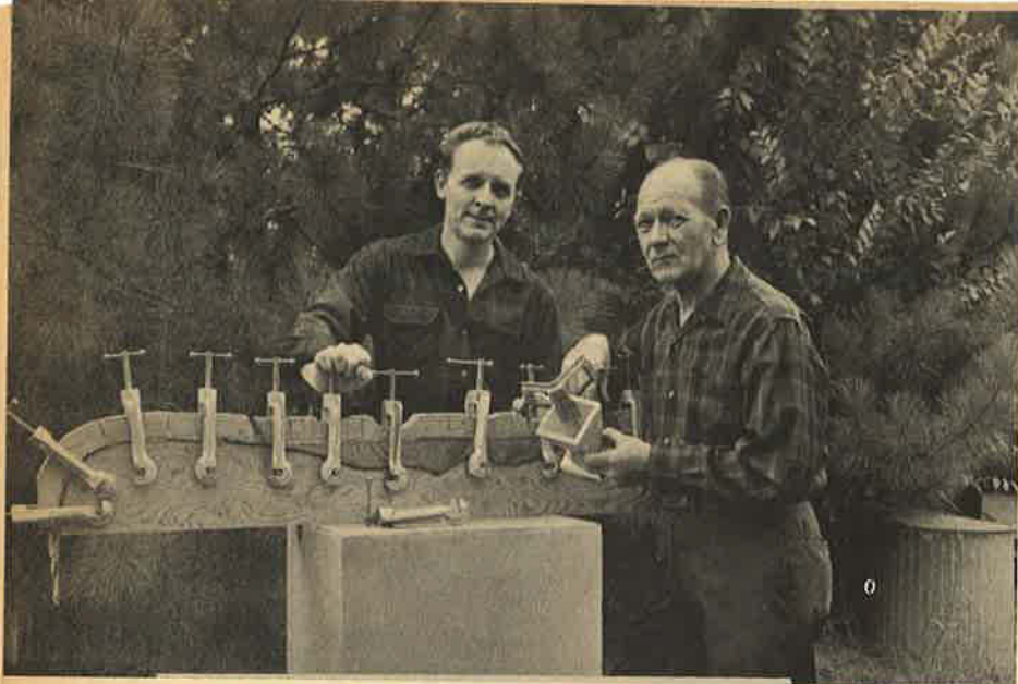
Koresh (left) and Frydenlund, with corner clamp, demonstrate the use of the bow clamps for laminated bows.
