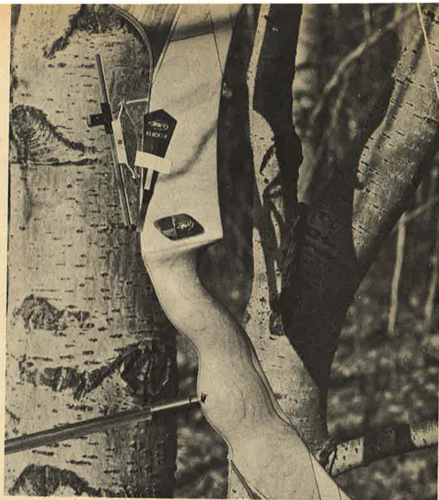
Roberts bow was equipped with sight by Reynolds, but Higgins attached a klicker and bubble level on his own.
