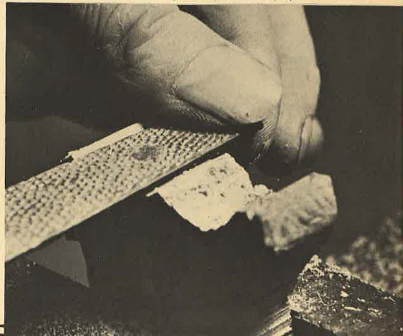
Using half-round side of wood file, smooth out the finger grooves, as you shape them to fit your own hand.
