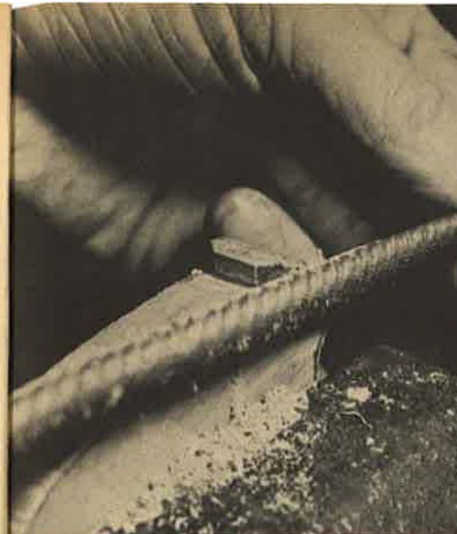
After basic form of hook has been cut out, use a rat tail file to cut arrow nock groove along the side. Use a forward and downward motion of file.
