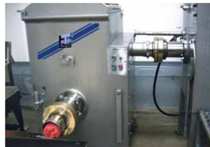
Standard 4000 Model 15 kW - 2 Speed Mince - 56 Head Gemini Connection - available to various machines
