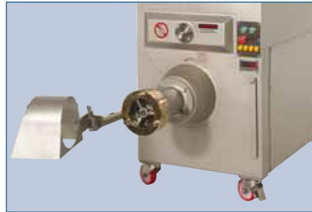
Illustrating 4200 Frozen 4 Speed Inverter Feedscrew Controller with Digital Readout
