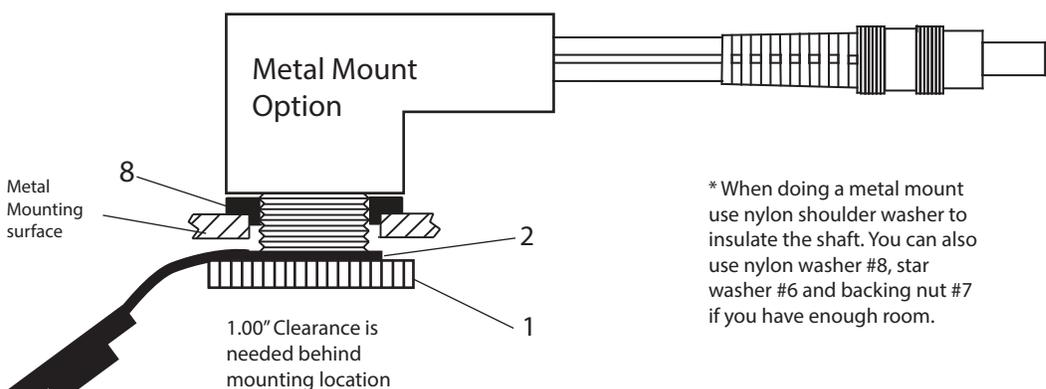
\*When doing a metal mount use nylon shoulder washer to insulate the shaft. You can also use nylon washer #8, star washer #6 and backing nut #7 if you have enough room.
