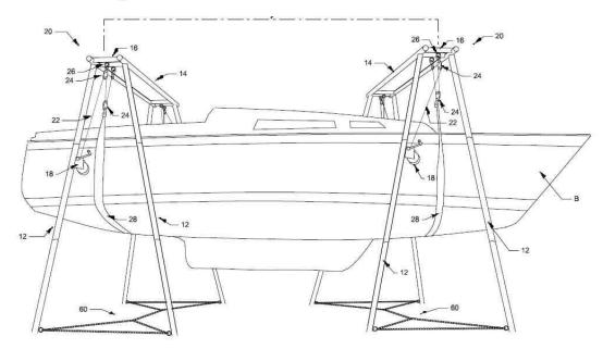
The image above show the lifting straps centered over each hoist from the side. As the images from page one show the straps can be slightly angled inward from bottom to top.
