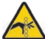
Pinch Point Hazard SAX392 SAX393
