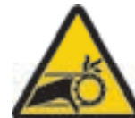
Chain Drive Entanglement Hazard SAX396 SAX397
