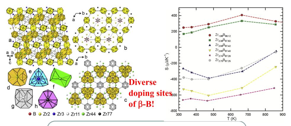
Excellent (S>200 µV/K) p-type or n-type in a material with a single crystal structure and composed of the exact same relatively abundant elements
