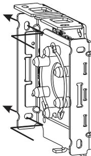
2. Install the motor end of the shade first and then the idler end when installing the motor into the side insert, You feed the wire of the motor through any of the gaps in the motor support posts where desired. (The shades should not be supported by the motor alone as this could cause damage to the motor. The installation team should support the shade as it is being completely inserted into the bracket set.)
