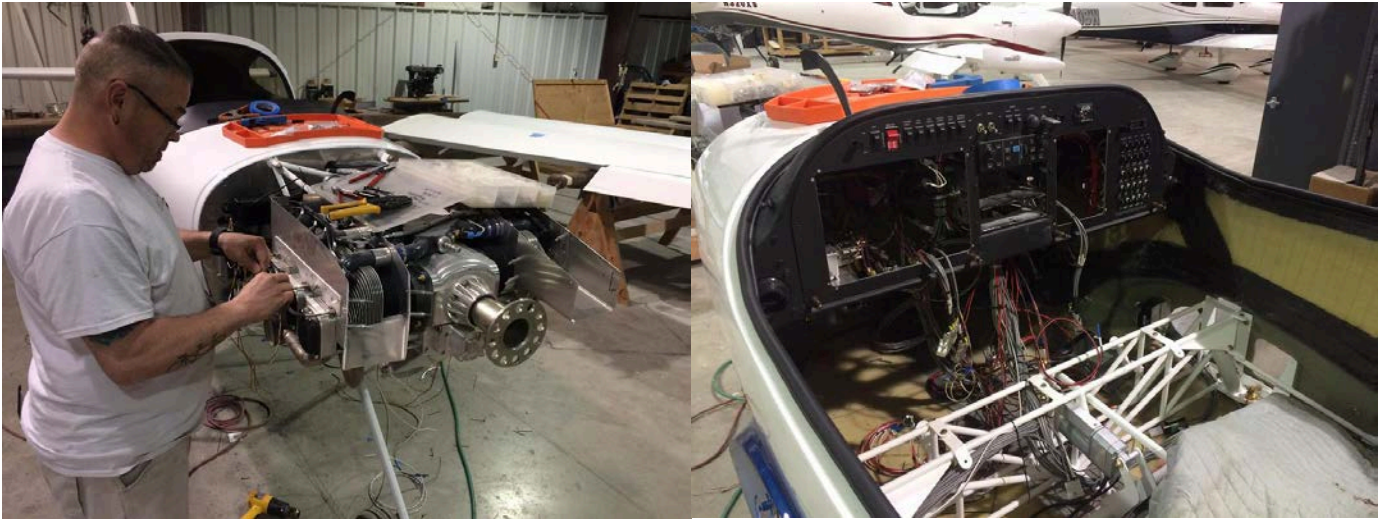
Jason Wiring the Engine and the Avionics Install (G3X)
