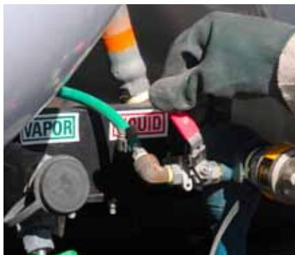
**Dual 1,000-gallon NH<sub>3</sub> tanks have improved efficiency for Southwest Family Farms of Plains, Kansas. A ball valve bleeds NH<sub>3</sub> from plumbing that joins the two tanks.**
