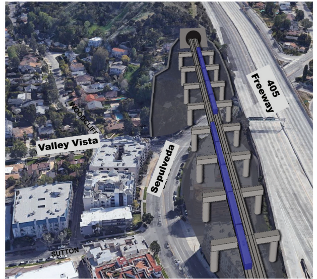
Alternative 4 Elevated Trains Demolish Hillside, Residences, and Businesses
