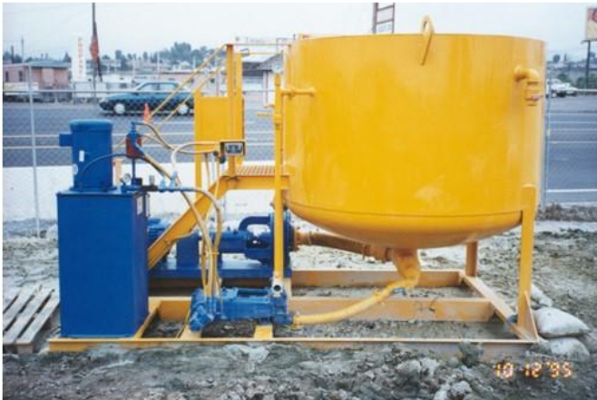
0-30 GPM, 0-200 psi with 750 gallon mixing/storage tank
