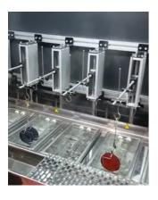
Easily adjustable elevator for degraded tintina. Customizable size and position for the desired degrading level.
