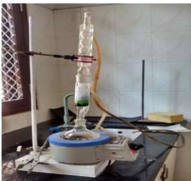
Fig. 1. Herbal extraction using Soxhlet apparatus
