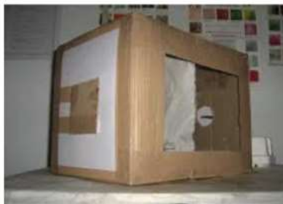
Fig. 2. Mosquito repellence test setup
