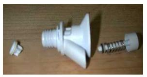
To make this into a bulkhead fitting, we need to run a piece of tubing through the spigot body in a water-tight way. For good flow-rate and resistance to clogging, I used the ubiquitous 3/8"OD copper tubing from Home Depot. The spigot body has a hole straight through it that the core used to be in. The hole is too small for the 3/8" tubing, but the spigot body has enough material that we can enlarge the hole just enough to get a tight fit. I just used a 3/8" bit in the drill press:
