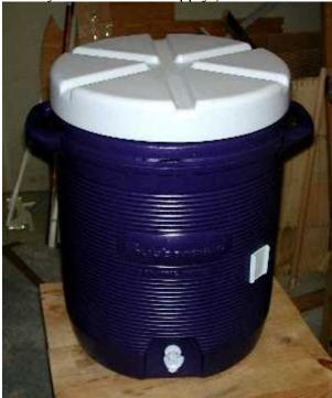
I ran the wort line out the spigot hole at the bottom, like everyone else. You have to remove the spigot. The spigot is held on with a large plastic nut on the inside, and a rubber gasket.
