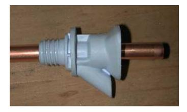
At this point, I replaced the spigot on the cooler, with the original rubber gasket and plastic nut. Filled with 10 gallons of water, it was water-tight. Nevertheless, to be extra sure, I applied some food-grade sealant around the joint on the inside.
