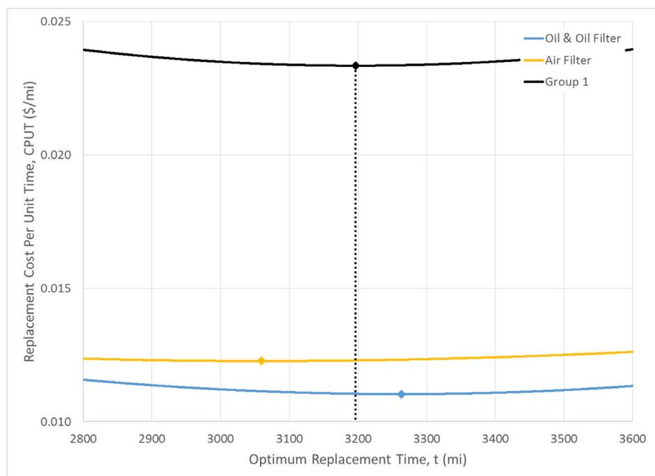
FIGURE 3 – OPTIMUM REPLACEMENT TIMES FOR GROUP 1 AND EACH COMPONENT IN GROUP 1
