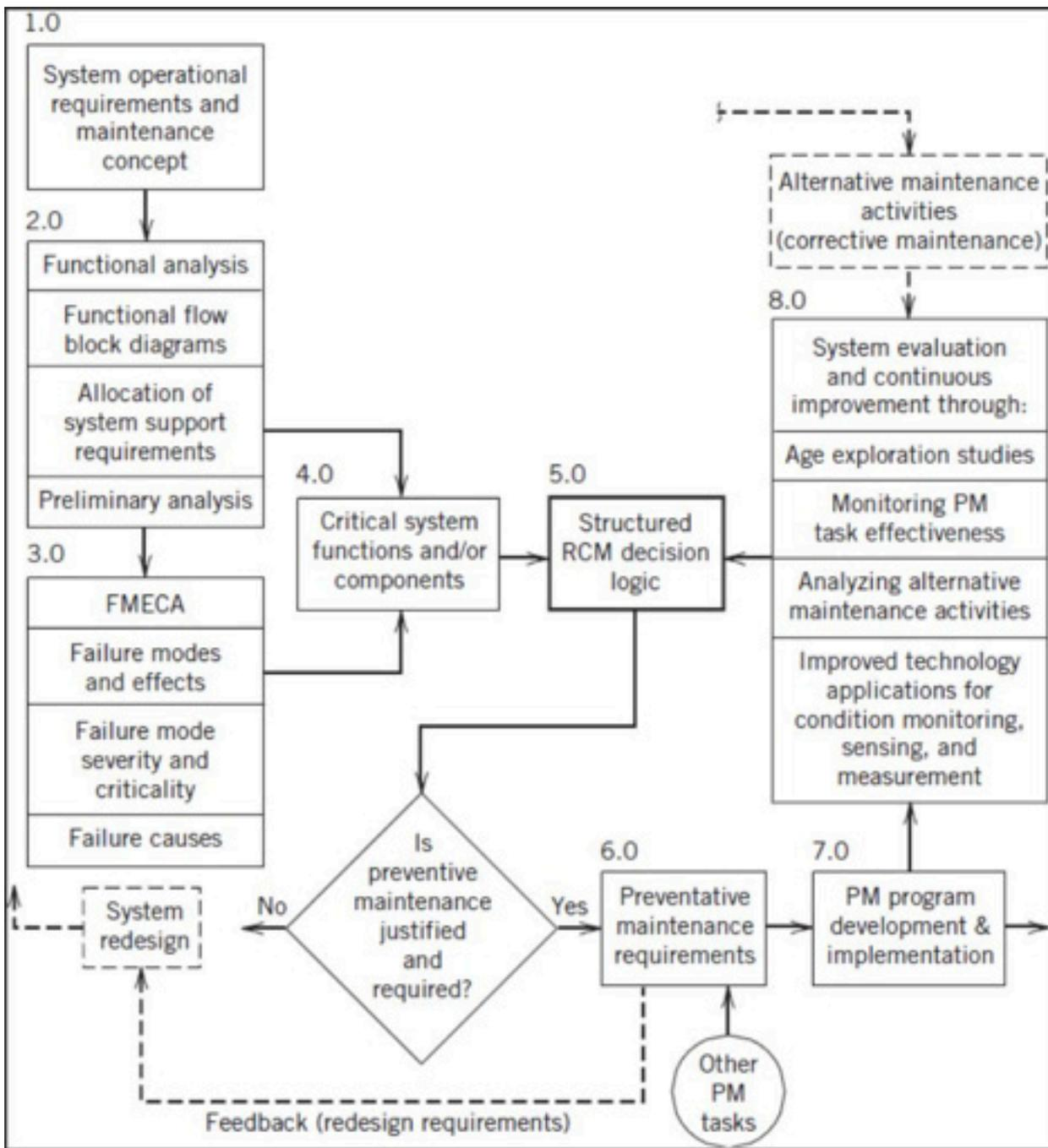
FIGURE C.11 – RELIABILITY-CENTERED MAINTENANCE ANALYSIS PROCESS
