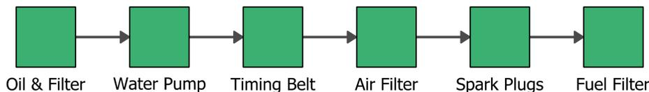
**TABLE 5 – RELIABILITY BLOCK DIAGRAM REPRESENTING THE SIX COMPONENTS IN THE SYSTEM FOR WHICH PREVENTIVE MAINTENANCE WILL BE PERFORMED**
