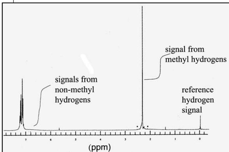
**Figure 3: High resolution NMR FFT signals from Toluene**
