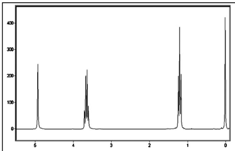
**Figure 6: High Resolution NMR FFT Signal from Ethanol**
