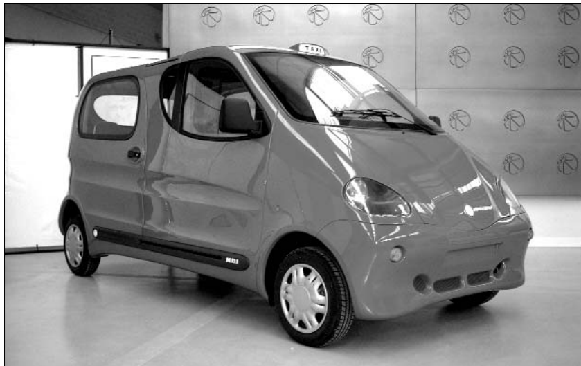
This car, built by French inventor Guy Nègre, runs on compressed air.
