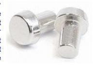
**Silver Cadmium Oxide (AgCdO)** has been popular for perhaps 50 years, particularly for its very good performance when switching inductive and motor loads. Contact material erosion is lessened and in particular, the material has an improved resistance to contact welding under conditions of short-term high peak inrush currents that result from switching large contactor coils, incandescent lamps and small motors.
