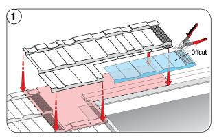
Cut the overhanging portion of the panel where it intersects with the stepped fascia as shown.
