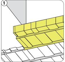
Measure, cut, and fold up panel 2" min. from the back of the panel to the front of protrusion.
