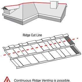
Measure, cut and install panels across ridge. Fasten as field panels. Overlapping panels is acceptable at the "horizontal" center line.
