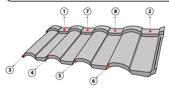
The fastening pattern for BARREL-VAULT Tile uses four (4) fasteners across the front nose down-turn and four (4) across the back up-turn of each panel.
