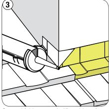
Cut and fold up panels 2" at sides of protrusion. Seal corner laps as shown.
