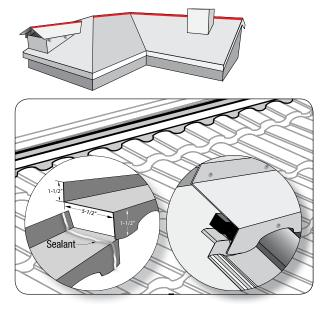
Apply a bead of Sealant between two overlapping Top Row pieces.
