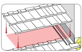
Cut out or fold-up nose of panel where Underpan metal exits onto lower panels. This allows water flow to exit the side-wall Underpan and onto the roof panels below.
