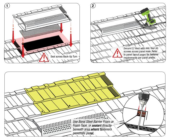
Top panel fastening is acceptable behind Boral Steel EZ-Vents, Chimney's & Skylights as long as they are positioned out of the main water channels on the high ribs of the panel. Fasteners should be covered with material from a Boral Steel Touch-Up Kit.
