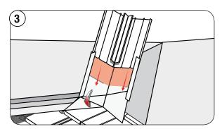
Install Valley metal over and onto the stone coated Flat Sheet. Apply a bead of sealant across the top of the Flat Sheet and embed the Valley into the sealant.
