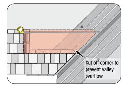
Measure, mark & cut panels to fit tightly against Valley center (reverse 'V'). Fasten valley section panels to roof decking similar to the other panels without penetrating valley flashing.
