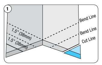
Mark cap as shown at center point. mark lines with 1.5" (38 mm) of spacing.
