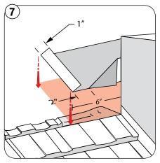
Install chimney saddle metal at back of chimney as shown. Extend saddle metal a minimum of 4" past each side of protrusion. Wakaflex<sup>®</sup> may be used as an option to form a chimney saddle around roof protrusions.
