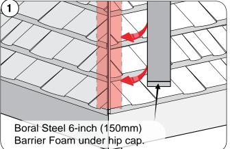
After cutting and installing panels to the Hip center-line, and creating a Hip Starter piece, apply Barrier Foam Roll (6" x 1" x 240") or butyl tape down center of hip, making sure the tape is seated on the panel surface at each panel course step.
