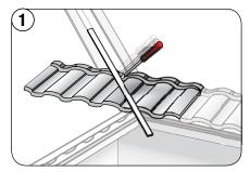
Measure, mark and cut panels to fit tightly against Valley center (reverse 'V').
