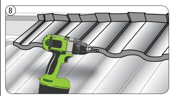
Fasten Ridge panel using four (4) fasteners across the nose (Refer to panel layout pages).
