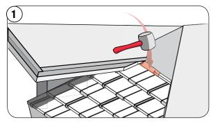
Flatten back flange against the roof deck.
