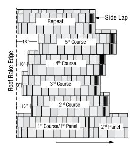
**Side Lap:** Grooved right-hand side of the panel is the "Under-Lap" portion and is covered by the "Over-Lap" of the next full panel on the same row.
