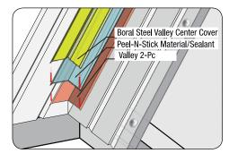
After all valley cut sections are installed, install a strip (min. 4" (100 mm) wide) of Peel-N-Stick type material or Sealant over the center seam as shown.
