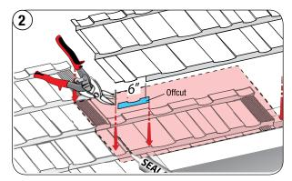
Lap the first cut-panel with a new full panel and cut/remove the section and seal as shown.
