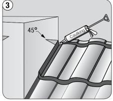
At back of chimney, seal each top corner section. Keep panel battens away from saddle as shown.
