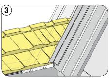
Valley panel cut & notched sections are fitted into the Valley 2-Pc as shown.
