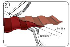
Mark the bend line 1½" in from the cut line (1" bend down when istalled batten-less).
