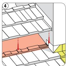
Install subsequent panels with a 2" bend up against the protrusion.
