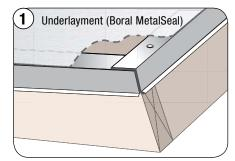
Install Drip Edge across fascia and up rake edges, when using Rake Channel. Install underlayment (Boral MetalSeal) on top of Drip Edge, as shown.
