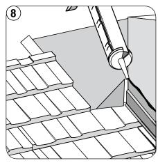
Install and seal Z-Bar flashing metal over folded sections as shown.
