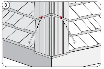
Fit and fasten each cap through the nose 2.5" (64 mm) from the outside edge of the cap.
