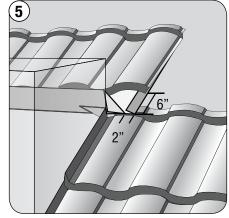
Apply a bead of sealant across Foam and 'seat' back cut-section panel onto Foam. Panels are to be fastened through front down-turn flashing, Foam and saddle into decking.
