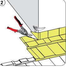
Cut a 45 degree angle as shown and fold tabs around protrusion.
