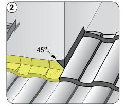
Cut 45° angle and fold tabs around chimney.
