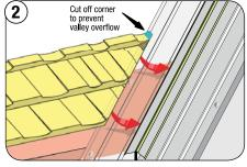
Notch the top Back Flange corner prior to fitting into the Valley.
