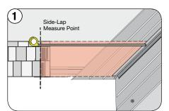
Measure from the Side-Lap reference point, mark & cut panels to fit into the Valley 2-Pc, matching the angle of the Valley.
