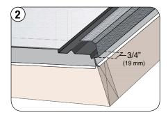
Install the Rake Channel up the rake extending it past the fascia Drip Edge by 3/4" (19 mm). Make sure the 'Locator-Lip' is snug against the rake Drip Edge and fasten with washer & grommet screws or apply sealant to screws.
