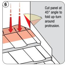
Flatten the back flange of the panel intersecting the top of the protrusion.
