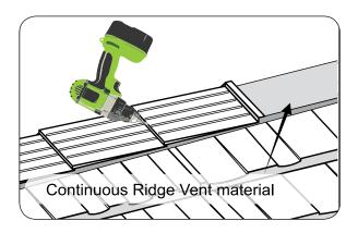
Cap fasteners to be 2.5" (64 mm) in from the outside edge of the cap and installed through the nose of each cap, through the foam/sealant/continuous Ridge Vent beneath & into the roof deck.
