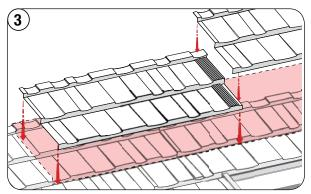
Apply either a bead of sealant, Barrier Foam or Foam Tape along the top surface of the under panel. Then install additional full panels half-lapping onto lower panel as shown.
