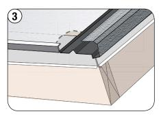
Install Gutter Riser across the fascia, underneath Underlayment and butt up against the Rake Channel and Valley pans.
