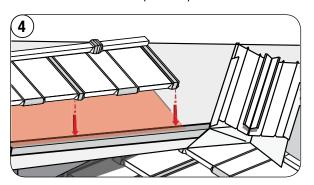
Then install the panels regularly as valley cut sections into the Valley 2-Pc.
