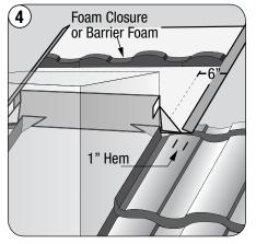
At back of chimney, install chimney saddle as shown. Extend saddle a minimum of 4" (100 mm) past each side of chimney. Hem ends 1" (25 mm) to keep water on saddle flashing.
