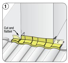
At front of chimney, measure, cut and fold up panel up 2".
