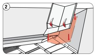
Form the stone coated Flat Sheet as an extension and exit tray for the upcoming valley. Apply sealant under the Flat Sheet where it exits on top of the panel beneath.
