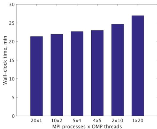
**Figure 5.** Wall-clock time of twenty source modeling vs. different MPI/OpenMP combinations within a single compute node.
