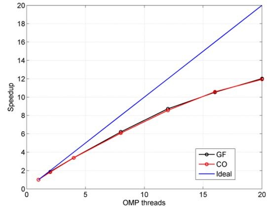
**Figure 3.** Speedup versus OpenMP threads used for GF and CO preconditioned BiCGStab.
