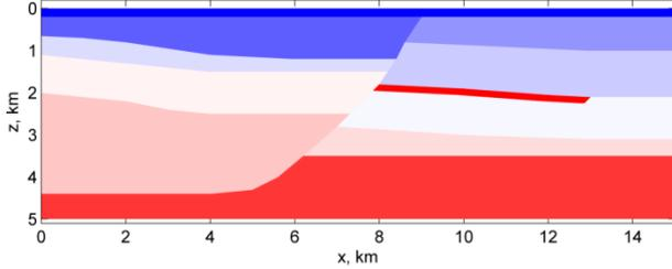
**Figure 1.** Marine resistivity model involving a host medium and 3D hydrocarbon deposit. The host medium is homogeneous in the  $y$ -direction.
