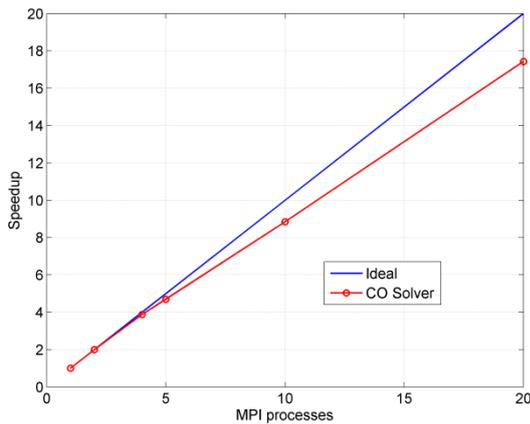
**Figure 4.** Speedup in modeling of 20 sources vs. number of MPI processes used, pinned to separate cores of a single compute node.
