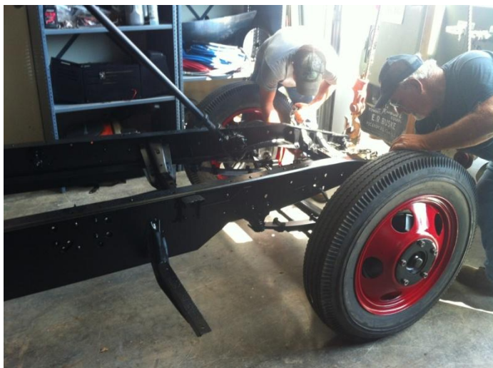
Directorate of Logistics employees preparing the fire truck's chassis for reassembly.
